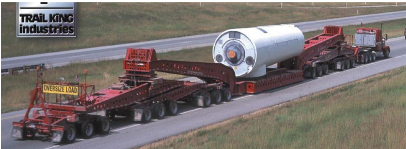
The trailer shown below is a Trail King 19 axle trailer hauling a nacelle for a wind turbine. Note that this trailer has tridam axles (three axle group), and probably would not be used in the Western States. Note that the nacelle weighs 192,000 lbs.
